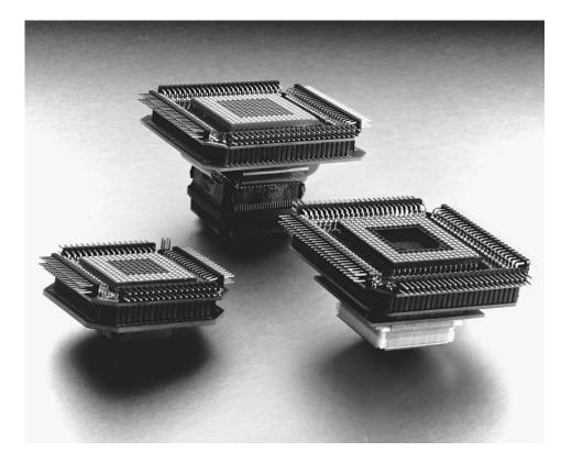
It provides hardware connection for testing, logic analysis, and emulation.
